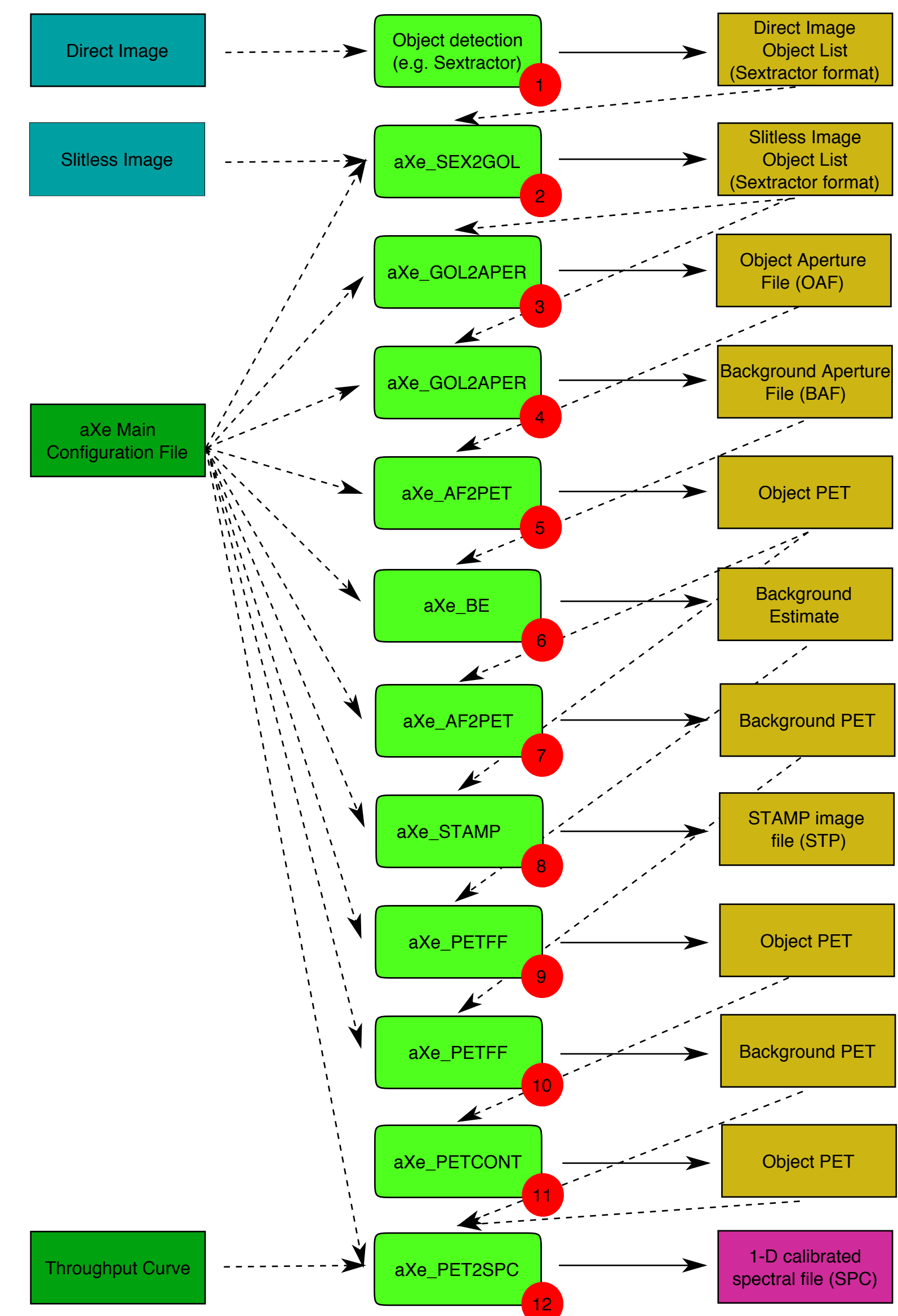
Figure 1: aXe tasks and a typical extraction process
