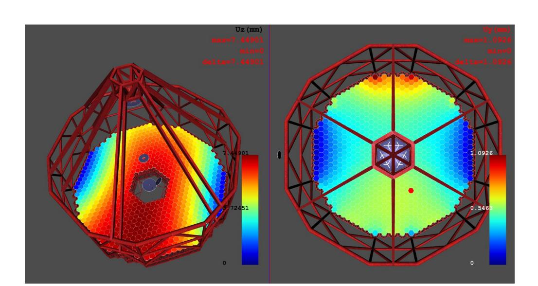
Fig. 3 FEM results. Deflection of Segmented mirror
