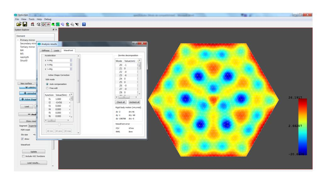
Fig. 10 Segmented mirror wavefront analysis
