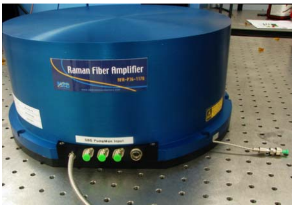
Figure 12: Left: picture of the RFA as delivered from MPBC; Right: spectrum of the emitted line taken with an IR Optical Spectrum Analyzer, at RFA power of 34W. The line profile asymmetry is due to the spectrum analyzer misalignment.
