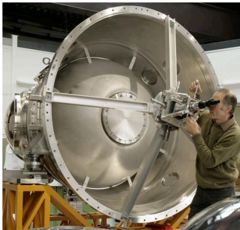
Figure 4: An example of alignment set up on HAWK-I. It consists in a sighting telescope mounted on a five axes adjustment mount which legs are interfaced on the instrument flange. The flange being the reference to define the instrument optical axis, we must align first the sighting telescope perpendicular to it. This is achieved by using an auto-collimation mirror installed on the flange and rotating the telescope mount by steps of 90 degrees with respect to the flange.
