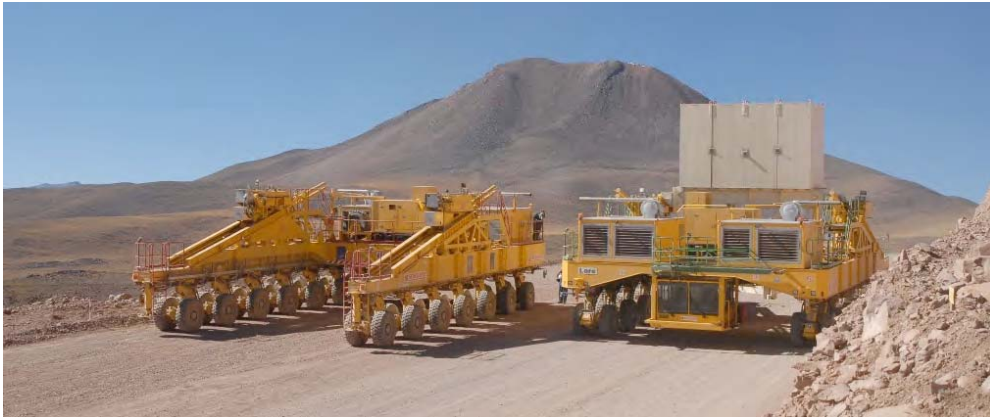
Fig. 6. Antenna transporters at a passing place on the road between the OSF and the AOS. The one on the right is carrying a dummy load which simulates the mass and physical interface of an antenna.
