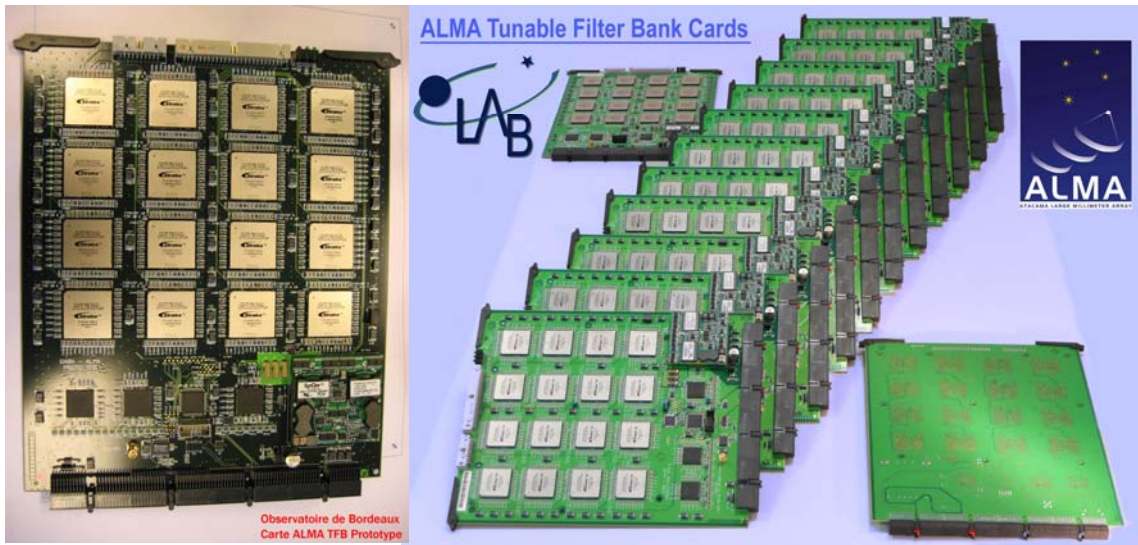
Fig. 10. Digital Filters used to provide flexible selection of spectral windows. Left: prototype Board. Right: Production.
