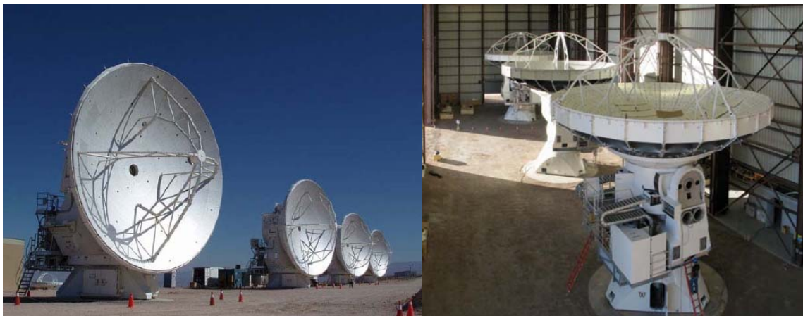
Fig. 5. Antennas at the OSF. Left, the four 12-m antennas from MELCO, and right, three of the five Vertex antennas on site at the time of writing.
