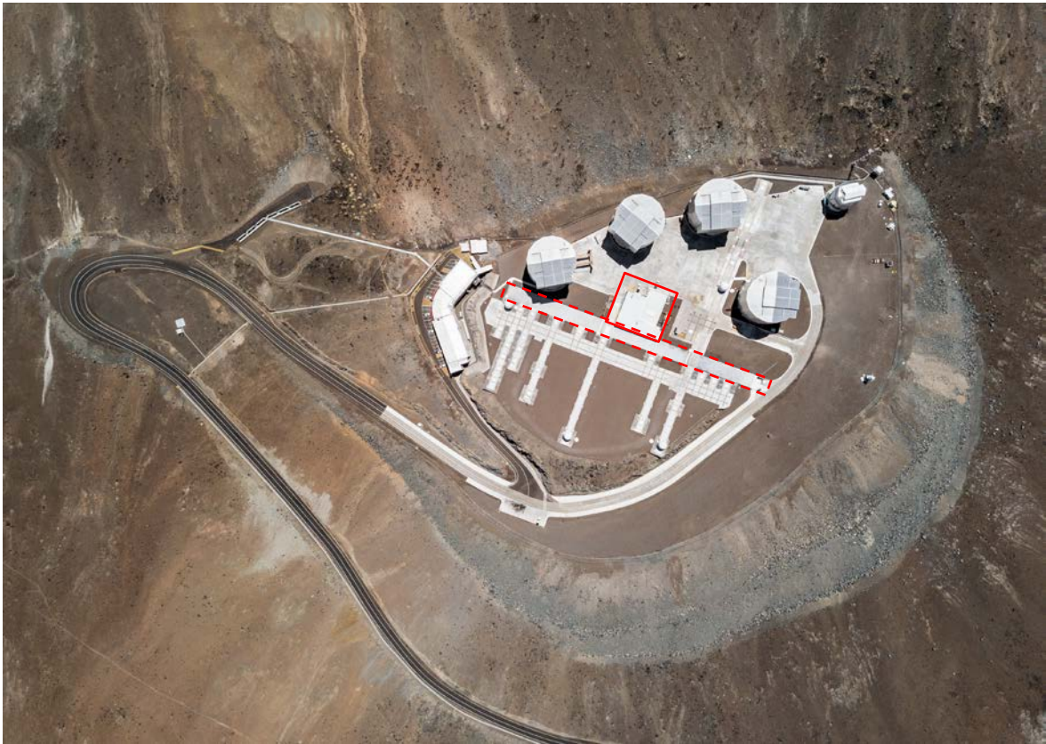
Figure 2: Paranal platform - the VLTI complex is shown in red, it includes the tunnel in red dashed line.
