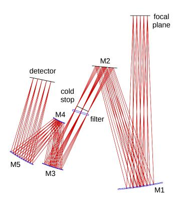
Figure 7: The optical path of the imager with a pixel scale of 0".045 is shown from the focal plane down to the detector.
