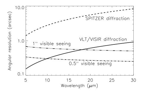
Figure 3: VLT diffraction limit (full line) versus seeing. The Spitzer Space Telescope diffraction limits (dashed) are shown for comparison. The Roddier dependence is shown for two optical seeings (dashed-dot).
