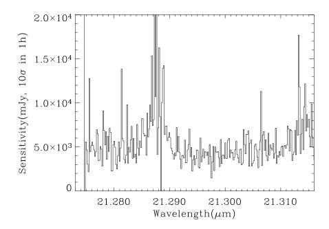
Figure 26: Observed sensitivity measured for the old DRS detector as a function of wavelength for high resolution mode (VII). Offered sensitivity is typically a factor of 2 larger and still valid until new measurements are available.
