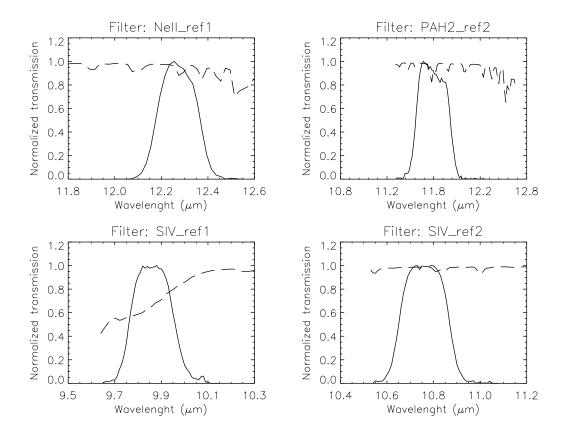
Figure 19: Transmission curves of VISIR imager filters, manufactured by OCLI. Overplotted (dashed) is the atmospheric transmission at low resolution. Only relative transmissions have been determined; their values are normalized so that their peak transmission is equal to 1.
