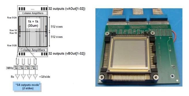
Figure 12: Left panel shows the AQUARIUS multiplexing readout scheme. Right panel shows the detector mounted in its socket.
