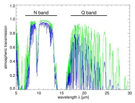
Figure 2: MIR atmospheric transmission at Paranal computed with ATRAN (Lord 1992, NASA Tech. Mem. 103957) for an altitude of 2600 m: in green for 1 mm of precipitable water vapor (PWV) at zenith (airmass = 1); in blue for 3 mm of PWV and airmass = 1.5. The largest changes are in the Q-band and at the edges of the N-band.
