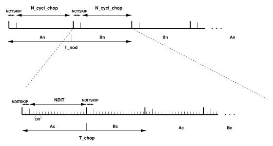
Figure 15: Data timing in VISIR. Ac and Bc refer to the two chopper positions, An and Bn refer to the two nodding (telescope) positions. Note the AnBnBnAn cycle sequence for the nodding to save observing time.
