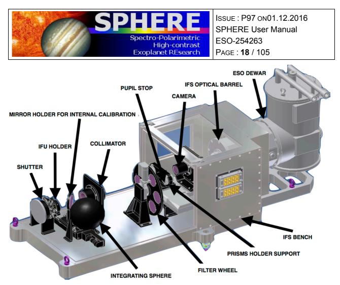
Figure 4: Inside the IFS. Note that the IFS optical bench is not cold, and that it has its own Lyot stop and internal calibration sources.
