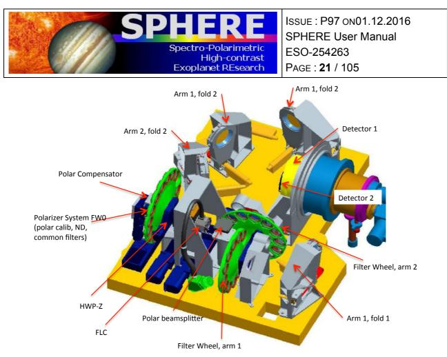
Figure 7: ZIMPOL schematic view showing the main elements of this visible polarimeter, from polarization compensator, common filter wheel, Ferroelectric Liquid Crystal (FLC) modulator to the splitter, filter wheels 1 and 2, and the two detectors.
