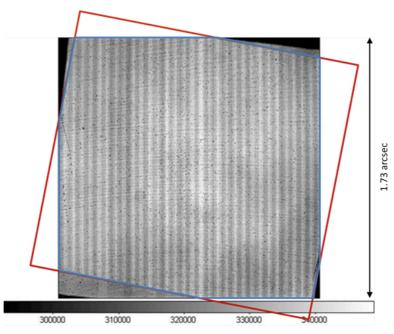
Figure 5: IFS flat-field and projection of the sky on the BIGRE detector (red) and ~1.73" x 1.73" FOV (blue).
