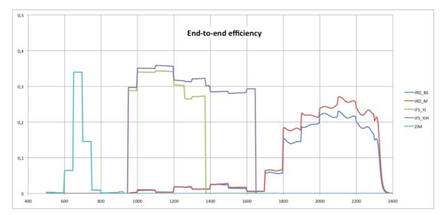
Figure 25: Transmission (as above) with different beamsplitters. In visible: separation between WFS and ZIMPOL uses a dichroic sending more light to ZIMPOL but in R band only; in NIR: the IFS/IRDIS dichroic 'K' feeds IFS with the its full Y-H range, with lower efficiency for IRDIS in K band only.
