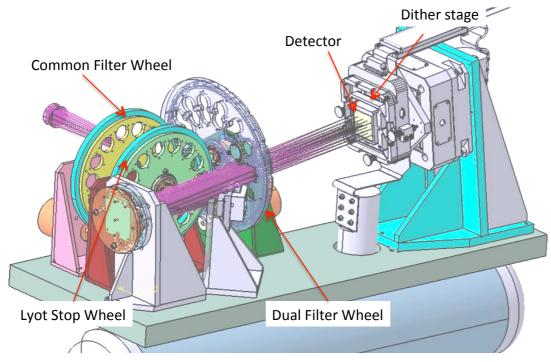
Figure 6: Inside view of the IRDIS cryostat. The CPI beam comes from the left, goes through the common filter and Lyot stop wheels, is split in two, then goes through the dual filter wheel before landing on the infrared detector.
