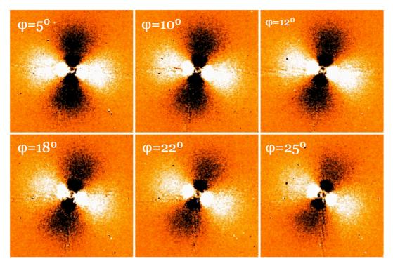
Figure 23:Effect of the instrumental polarization (efficiency loss due to increased crosstalks at a varying derotator angle). The « butterfly pattern » rotates with time and its signal to noise ratio decreases significantly. This is the polarimetric signature of a bright face-on disk (H-band observations).
