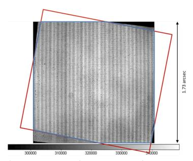
Figure 5: IFS flat-field and projection of the sky on the BIGRE detector (red) and  $\sim$ 1.73" x 1.73" FOV (blue).
