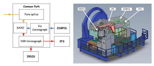
Figure 1: SPHERE sub-systems (left) including the common path (CPI) with adaptive optics system SAXO, coronagraphs, and sub-instruments IRDIS, IFS and ZIMPOL. Left: schematic view of the instrument on the Nasmyth platform.
