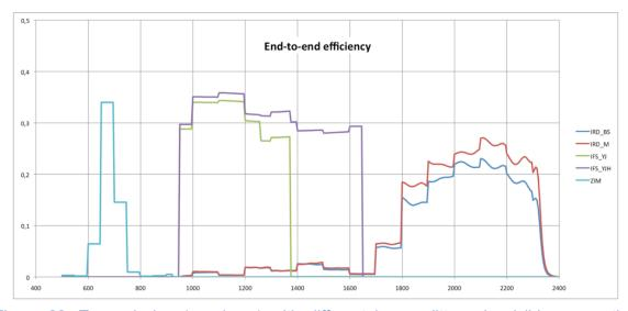
Figure 22: Transmission (as above) with different beamsplitters. In visible: separation between WFS and ZIMPOL uses a dichroic sending more light to ZIMPOL but in R band only; in NIR: the IFS/IRDIS dichroic 'K' feeds IFS with the its full Y-H range, with lower efficiency for IRDIS in K band only.
