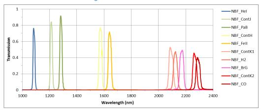
Figure 29: IRDIS NB filters.
