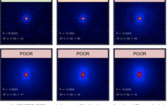
Figure 11: SPHERE PSF morphology and Strehl ratio as a function of R magnitude (see Table 7 and Table 8 for details).
