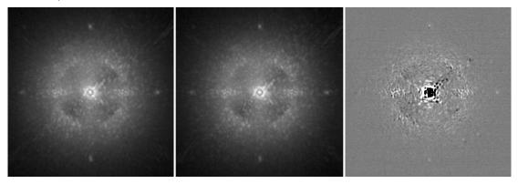
Figure 12: Coronagraphic images obtained in IRDIS H2 (left) and H3 (center) DBI filters, and the result of spectral differential imaging H2-H3 (right).
