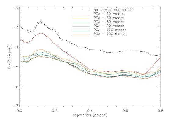
Figure 16: IFS  $5\sigma$  sensitivity on lota Sgr as function of angular separation, for different principal components retained in the speckle subtraction using both spectral and temporal diversity (ADI).
