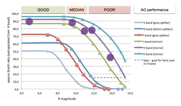
Figure 10: Theoretical and measured (purple circles) SPHERE-SAXO Strehl ratio as a function of R magnitude for good seeing conditions and different wavelength ranges from V to K (see Table 7 and Table 8 for details).
