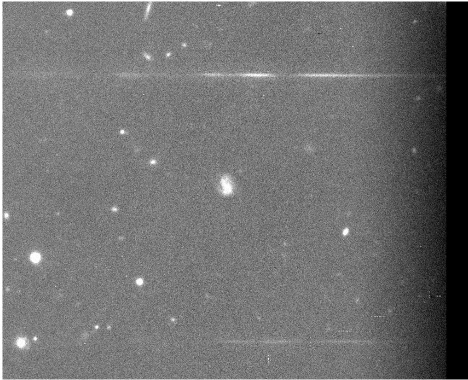
Figure 19: Example of reflection of light from a star (in this case, two stars to the West) outside the field. Such features can occur on each of the four corner CCDs.
