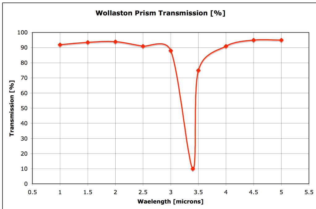
Figure 5-14: Transmission as a function of wavelength for the Wollaston prism. The big absorption feature at 3.4 microns is due to the resin material.
