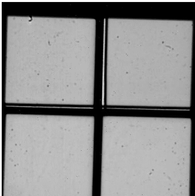
Figure 5-2: Flat field image of the SDI+ mode. The transmitted wavelengths are 1.6 mm (top left), 1.575 mm (top right) and 1.625 mm (bottom left and right).
