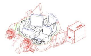
Figure 1: Cut through HAWK-I for an optical and mechanical overview. Blue: optical components; black: cold assembly, filter wheels, detector assembly; green: radiation shield; red: vessel structure, cryogenic components, electronic rack.
