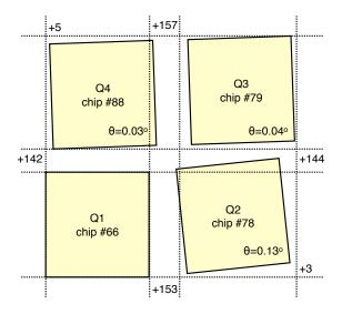
Quadrants 2,3,4 are tilted with respect to quadrant 1 by 0.13, 0.04, 0.03 degrees, respectively. Accordingly, the size of the gaps changes along the quadrant edges.
