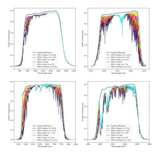
Figure 11: Effect of PWV on the transmission curves of Y-, J-, H-, and K-bands. The black curves denote the transmission curve without atmosphere effects, and the color curves represent the transmission curve convolved with the sky transmission at different PWV values. PWV=2.5mm is used as a reference value to compute the G (GAIN) value in the different PWV values.
