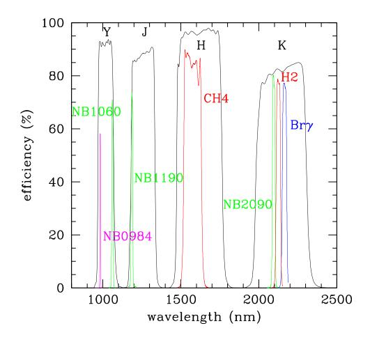
Figure 22: HAWK-I Filters. Black: broad-band filters Y, J, H,  $K_s$ , Green: cosmological filters NB1060, NB1190, NB2090; Red: CH4, H2; Blue: Br $\gamma$ ;magenta: visitor filter NB0984
