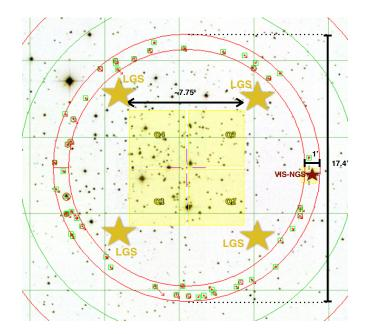
Figure 5: GRAAL focal plane illustration. The 4 LGS rotate with respect to the FoV and the lasers are side-launched. The visible TT-star selection annuli is shown. However, HAWK-I is offered in TTS-free mode only. So users can neglect that part.
