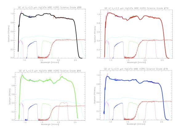
Figure 15: Quantum efficiency of the HAWK-I detectors
