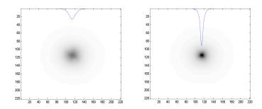
Figure 4: Observed PSF without (*left*) and with (*right*) GRAAL correction.
