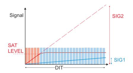
Figure 8: Saturation threshold for nondestructive sampling and extrapolation of detector signal for high flux levels. Only pixel values below SATLEVEL are taken into account for calculation of slope for pixels with high flux (red). For low flux pixels (blue) all nondestructive readouts indicated by rectangles are used.
