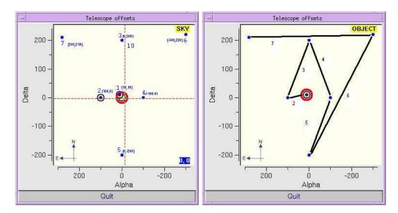
Figure 13: Left: Pop-up window at the start of an example template: it provides a quick check of your offset pattern. Right: Offset execution along the template.
