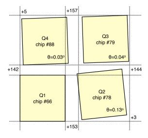
Quadrants 2,3,4 are tilted with respect to quadrant 1 by 0.13, 0.04, 0.03 degrees, respectively. Accordingly, the size of the gaps changes along the quadrant edges.
