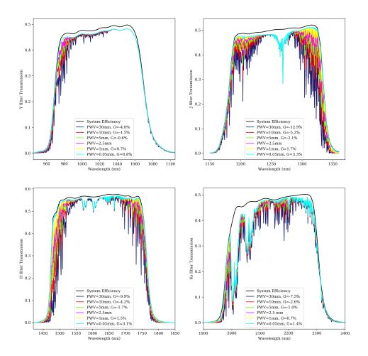
Figure 10: Effect of PWV on the transmission curves of Y-, J-, H-, and K-bands. The black curves denote the transmission curve without atmosphere effects, and the color curves represent the transmission curve convolved with the sky transmission at different PWV values. PWV=2.5mm is used as a reference value to compute the G (GAIN) value in the different PWV values.
