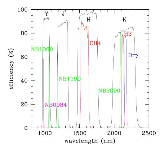
Figure 21: HAWK-I Filters. Black: broad-band filters Y, J, H,  $K_s$ , Green: cosmological filters NB1060, NB1190, NB2090; Red: CH4, H2; Blue:  $Br\gamma$ ; magenta: visitor filter NB0984
