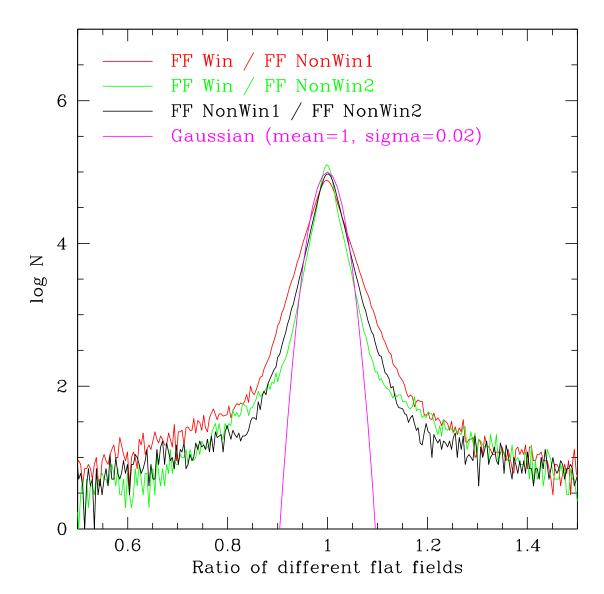
Figure 23: Histograms of the ratios between a windowed and two non-windowed  $K_S$  twilight flats. For comparison, the ratio of the two non-windowed flats and a Gaussian function is also shown.
