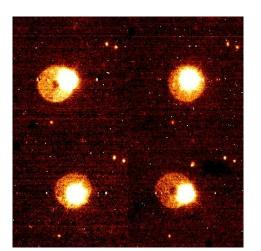
Figure 20: Smoothed enhanced images of the optical ghosts visible in the four quadrants for the NB1060 (left) & NB1190 (right) filters
