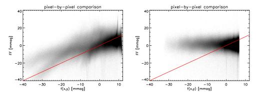
Figure 9. Pixel-by-pixel comparisons of f(x, y) with the flatfield (FF) used to process the images before fitting f(x, y). Left: master flat versus derived f(x, y), right: illumination-corrected flat versus f(x, y).
