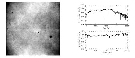
Figure 3. Co-addition of a selected sample of 240 *R* sky flats. *Left*: Image of the combined flatfield. The intensity scale range is 3%. *Right*: Traces along the central column (upper panel) and central row (lower panel).
