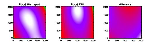
Figure 7. Comparison between the flatfield correction frames derived in the current work and FWII. Left: f(x, y) from FAP, center: from FWII, right: the difference. The colour scale in all three panels is identical.
