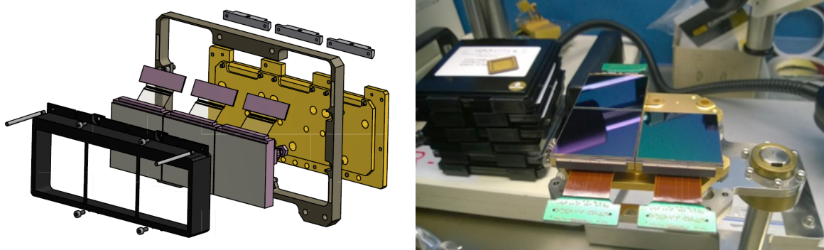
Figure 7: The 3 CRIRES H2RG detectors are shown (right) together with the detector mount (left)
