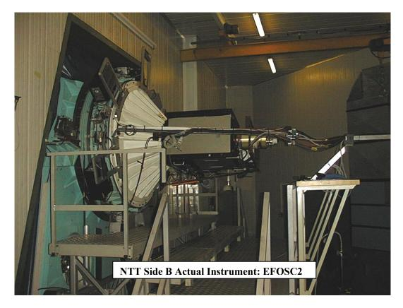
If the area is required for a Visiting Instrument, EFOSC2 and the conical adapter can be removed and stored in their supporting and handling frames.
