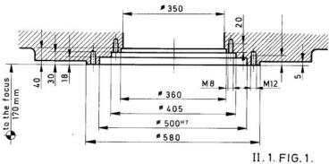
Maximum load possible to apply at its focus is **7500 N** (This figure has not been checked due to unclear information)
