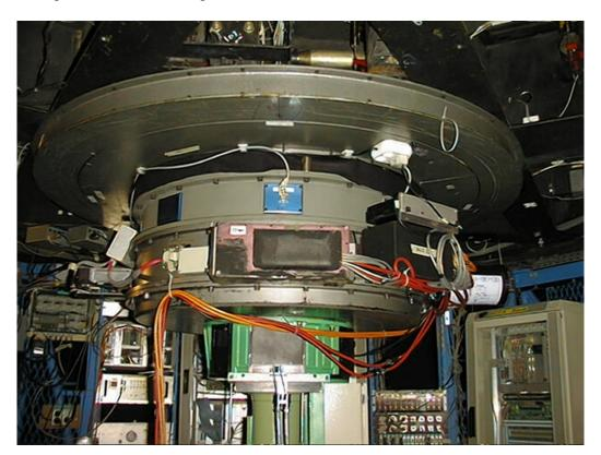
The available space from instrument flange to floor of the Cassegrain cage is 1500 mm and the free space around the telescope instrument axis is within a radius of 1200 mm. Any instrument should consider some free space of at least 100 mm from the above mentioned dimensions in order to allow the pass of cabling.
