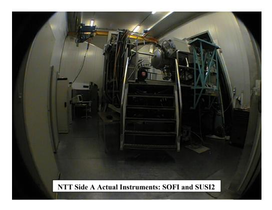
The actual available space is given by the displacement of SOFI by  $750\ mm$ , maximum possible within the fixed platform.
