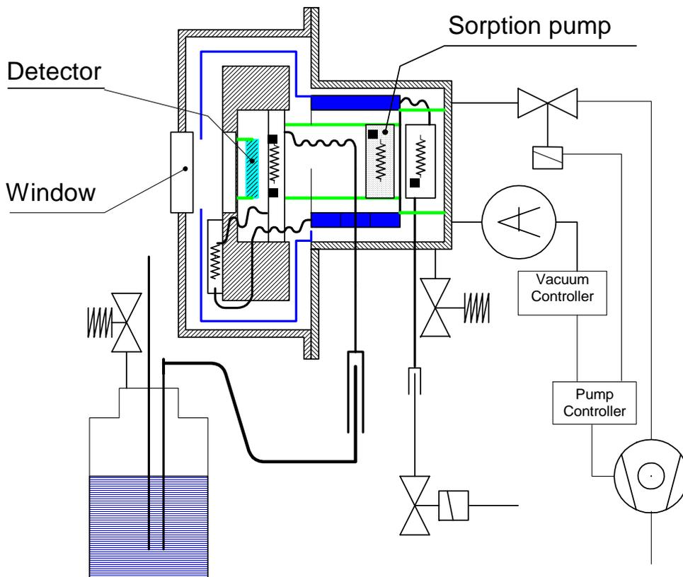
Figure 9 : Schematic of a CCD cryostat system
