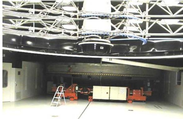
Figure 7: Overview of the coating facility with in the background the lower part of the vacuum chamber
