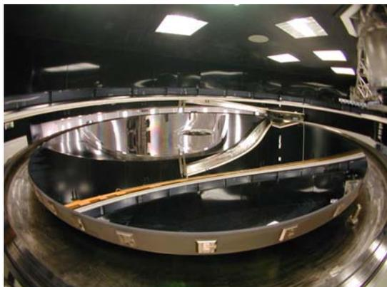
Figure 5: Primary mirror right after aluminization
