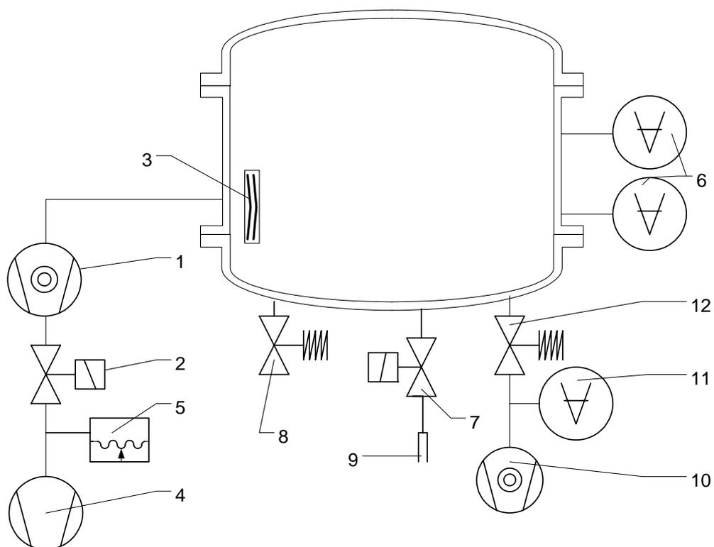
Figure 12: Vacuum schematic of a large IR instrument
