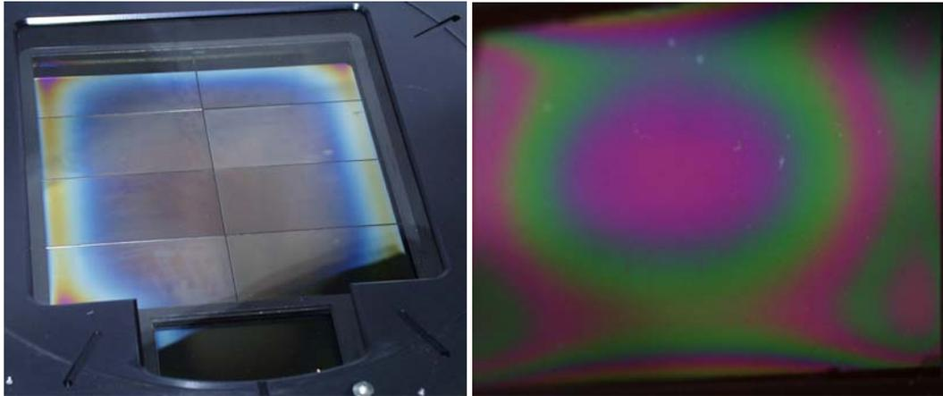
Figure 8: Contaminated CCD chips
