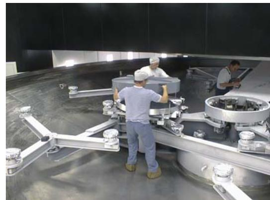
Figure 6: Preparation of small mirrors in the chamber
