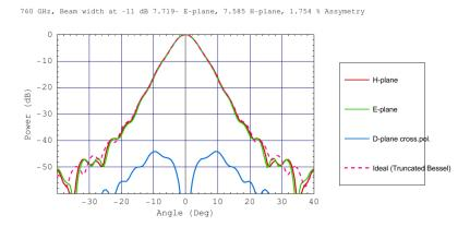
Figure 61: Similar data as in figure 60, but now for 760 GHz, which is beyond even the most extended RF band considered in this study.
