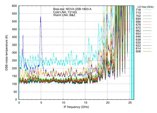
Figure 26: DSB noise temperature of the reference mixer as function of IF frequency, for 15 LO frequencies using the new bias-tee.
