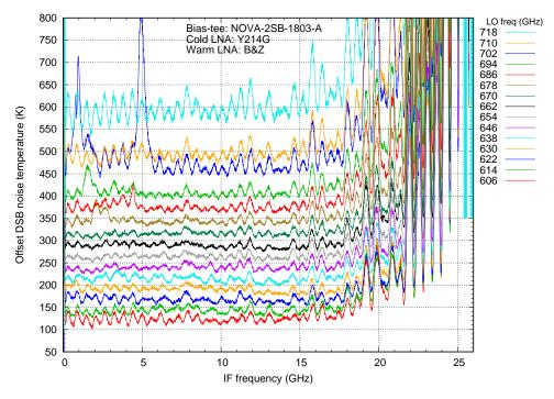
Figure 27: The DSB noise temperatures as function of IF frequency using the new bias-tee. Each curve offset vertically by a multiple of 25 K to separate them. The bottommost curve (606 GHz) is at the original level.
