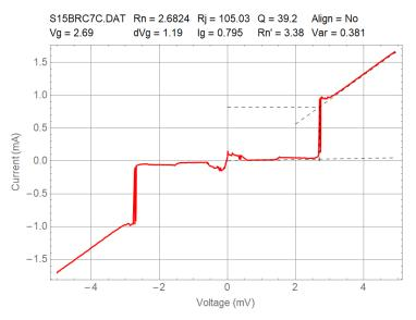
Figure 63: Example of measured I-V curve with key parameters (see figure 62) automatically determined.
