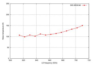
Figure 21: DSB Noise temperature of the used test mixer, as recently measured in ALMA Band 9 cartridge #99.
