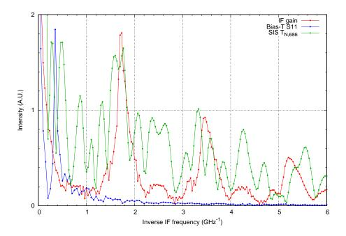
Figure 31: Fourier transforms of the IF gain (by shot noise), the input reflection  $(S_{11})$  of the bias-tee and the mixer noise temperature for one arbitrary LO frequency.
