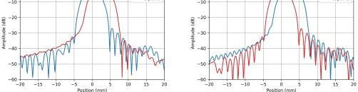
Figure 50: Orthogonal cuts of the P0 and P1 polarisation beams in the focal plane. The displacement of the E- and H-planes depends on the angle of the incoming RF beam, which is  $0.94^{\circ}$  with respect to the cartridge axis.
