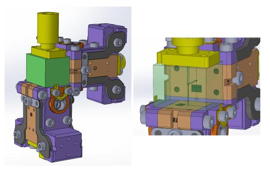
Figure 55: The basic geometry of two SEPIA Band 9 2SB mixers around a block (green) that could contain a Dunning-type OMT. On the right a detail showing the basic waveguide runs. The OMT structure itself is not drawn, but since it will be about 2 mm long, it will certainly fit in a block like this. The split will be in the vertical plane.
