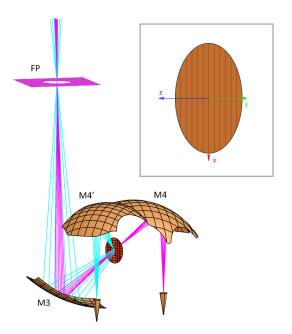
Figure 42: Model of the Band 9 optics as implemented in GRASP. Light blue rays represent polarization P0, which is reflected by the grid. Pink rays represent polarization P1, which is transmitted by the wire grid. The top-right panel shows an enlargement of the polarizing grid with its reference coordinate system.
