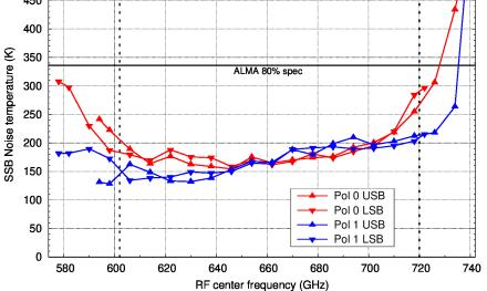
Figure 1: Single-sideband noise temperature integrated over the 4–12 GHz IF band for the delivered SEPIA660 Receiver (lab qualification data). The 80% (336 K) and 100% (500 K) "ALMA specifications" are simply the Band 9 DSB limits multiplied by two. Measurements performed at 4.0 K
