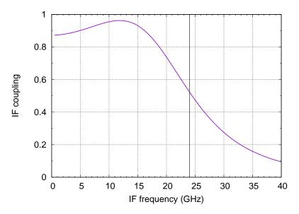
Figure 9: Simulated IF power coupling of the Band 9 SIS junction at the operating point.
