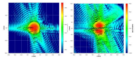
Figure 49: Co-polar (left) and cross-polar (right) beam computed in the focal plane at 661 GHz.
