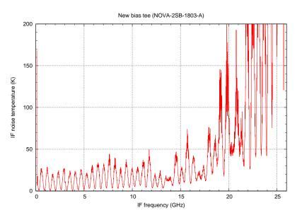
Figure 29: IF noise temperature measured by shot-noise method.
