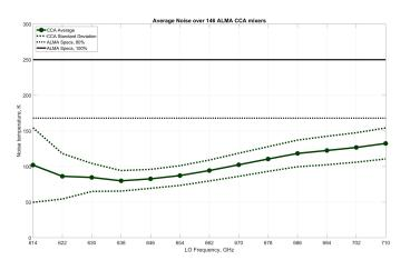
Figure 38: Average DSB noise temperature of mixers installed in the current Band 9 DSB cartridges.
