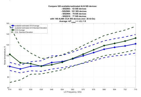
Figure 40: Average Noise temperature of 320 available and estimated mixers compared to the Band 9 cartridge average.
