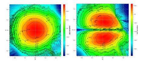
Figure 48: Co-polar (left) and cross-polar (right) beam computed in the far-field at 661 GHz.
