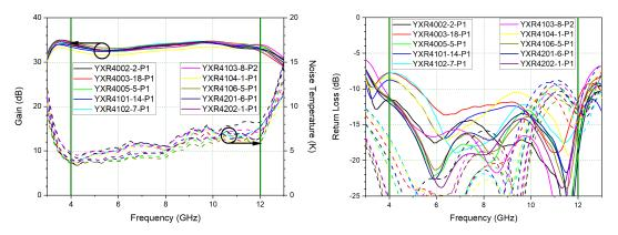
Figure 10: The gain and noise temperature (left) and the input and output matching (right,  $S_{11}$  solid,  $S_{22}$  dashed) of ten cryogenic Yebes 4–12 GHz LNAs (YXR4000 series). Eight of these have been integrated into the Band 9 2SB CCAs for SEPIA and LLAMA. Graphs courtesy of R.I. Amils Samalot, Observatorio Astronómico de Yebes.
