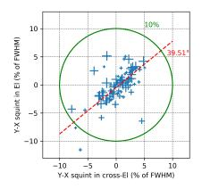
Figure 43: On-sky Y-X polarisation beam squint in cross-elevation vs. elevation coordinates in units of the beam FWHM at 661 GHz. The 10% limit is shown as a green circle and the red line is the fit to the measured data, which highlights a preferred angle of about  $39.5^{\circ}$ .
