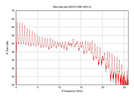
Figure 30: The IF gain measured by shot-noise method.
