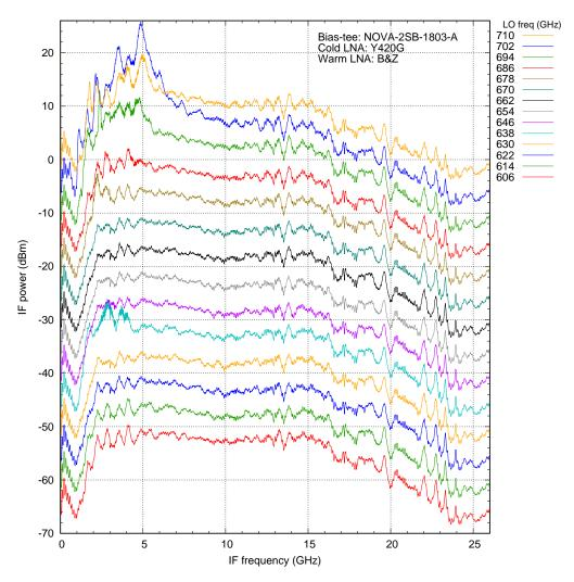
Figure 33: IF power for different LO frequencies using the new Yebes Y420G LNA, looking at a 300 K load. Each curve is offset vertically by a multiple of  $5 \,\mathrm{dB}$  to separate them. This result should be compared to the one shown in figure 28, taken with the previous generation of LNA.
