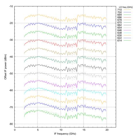
Figure 37: IF power for different LO frequencies for the 2SB mixer, looking at a 300 K load. Each curve is offset vertically by a multiple of 5 dB to separate them. Solid line: USB, dotted line: LSB.
