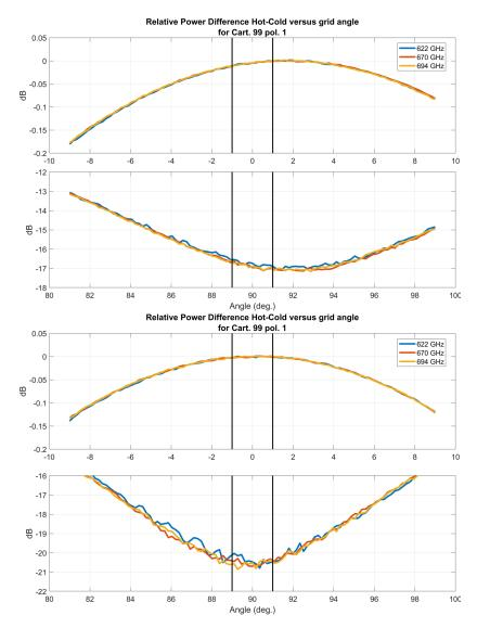
Figure 59: Co- and cross-polar level of the Band 9 optics with (upper pair) and without (lower pair) polarizing grid. The corresponding curves are normalized for  $0 \, dB$  at the co-polar maximum, so the minimum in the cross-polar curves immediately gives the best possible cross-polar level. Each curve was measured at three different frequencies, and no significant frequency dependence is observed.
