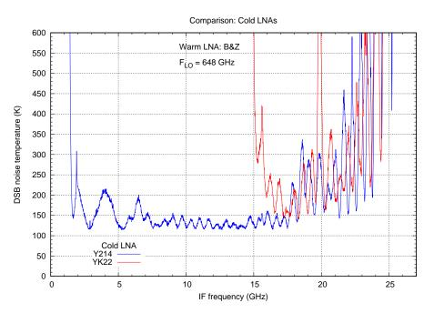
Figure 25: The DSB mixer noise temperature with both cold Yebes LNAs (Y214: 2–20 GHz, YK22: 20.5–24.5 GHz, nominally) and the old bias-tee.
