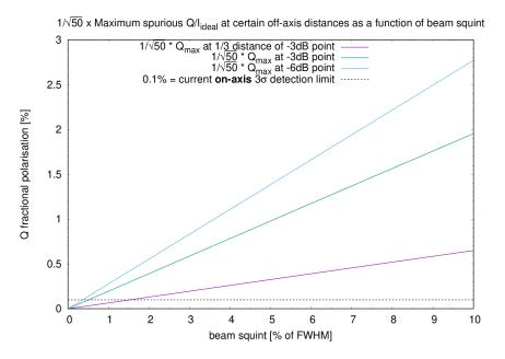
Figure 67: Spurious Q vs. beam squint
