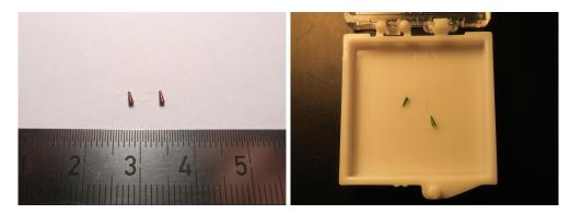
Figure 12: Photographs of the conical inductors of Coilcraft (BCL-122JL,  $1.2 \,\mu\text{H}$ , left) and Piconics (CC45T47K240G100,  $0.84 \,\mu\text{H}$ , right). These were provided by both suppliers as free samples.
