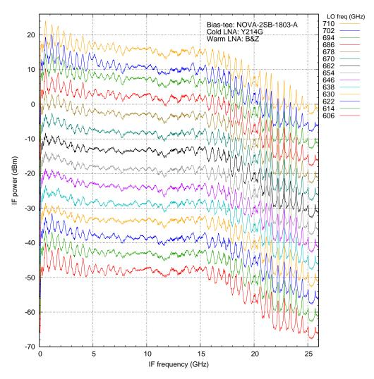
Figure 28: IF power with the new bias-tee and the Y214G LNA, and the mixer looking at a 300 K load. Each curve offset vertically by a multiple of 5 dB.
