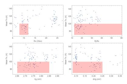
Figure 64: A noise temperature average over LO frequencies of NbTiN ALMA Band 9 mixers as delivered to ALMA as a function of automatically determined unpumped DC I-V parameters: top left  $R_n$ , top right  $R_j/R_n$ , bottom left  $V_g$ , bottom left  $\Delta V_g$ . Red shaded areas indicate regions of optimum performance which will be used for merit function.
