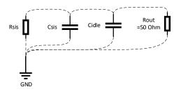
Figure 8: A representative equivalent circuit of the Band 9 SIS mixer in the IF domain.
