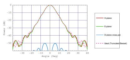
Figure 60: Calculated co-polar far-field intensity in E- and H-plane cuts, and crosspolar in a diagonal (D-plane) cut, for the original Band 9 feedhorn, obtained by propagating the field distribution in the mouth of the horn, in its turn obtained by mode-matching calculations. This example is for 660 GHz, the middle of the 600–720 GHz band.
