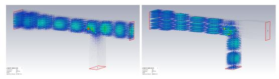
Figure 53: Simulated E-field distribution in the Dunning OMT for horizontal (left) and vertical (right) input polarization. The input (port 1) is on the left in each case, and the two outputs on the right (port 2) and the bottom (port 3).
