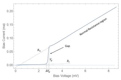
Figure 62: DC I-V curve of SIS junction with analysis parameters indicated as follows:  $R_n$  is normal resistance,  $V_g$  is Gap voltage,  $R_j = R_l$  is subgap resistance,  $\Delta V_g$  is width of gap region.
