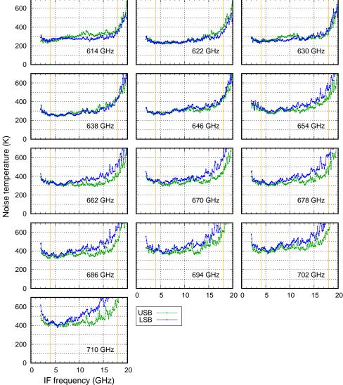
Figure 36: The SSB noise temperature of the 2SB mixer as function of IF frequency for different LO frequencies.
