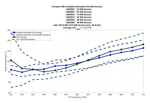
Figure 41: Average Noise temperature of 480 available and estimated mixers compared to the ALMA Cartridge average.
