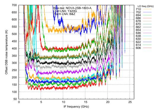
Figure 32: DSB noise temperature, as in figure 27, but with the new Yebes Y420G LNA. The measurement data (taken by spectrum analyser) looks more noisy than in the former measurement due to averaging over fewer SA sweeps. Also, in this measurement the mixer was clearly underpumped at several LO frequencies resulting in excess noise. Each curve from bottom to top is offset by 25 K from the preceding one (the 606 GHz curve is at its "native" level).
