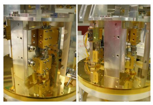
Figure 22: Left: one of the 4–20 GHz IF chains mounted in roughly the position of the former IF isolator in Band 9 CCA #99. The LNA is below, the bias-tee on top. Right: overview, with both IF chains visible.
