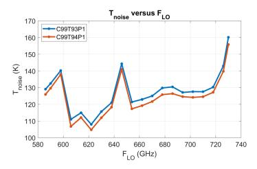
Figure 57: Noise temperature of an arbitrary Band 9 mixer measured with and without the polarization grid.
