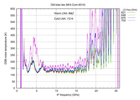
Figure 24: DSB noise temperature of the reference mixer as function of IF frequency, 4 LO frequencies using the old bias-tee.
