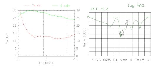
Figure 17: The gain and noise temperature (left) and the input matching (right) of the cryogenic 20.5–24.5 GHz LNA (YK22 005) used for some of the the ultra-wide IF DSB measurements, at low temperature. The axes of the right panel: horizontally 0–40 GHz, vertically 10 dB/div, 0 dB at the triangle on the right. Images courtesy of Observatorio Astronómico de Yebes.
