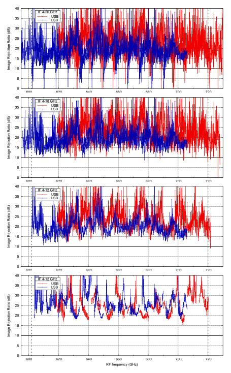
Figure 35: The combined IRR data for the tested mixer pair. Top panel: full IF range (4–20 GHz). Second panel: IF range 4–18 GHz. Third panel: IF range 4–12 GHz. Bottom panel: the same pair of SIS devices measured (over 4–12 GHz) during the SEPIA/LLAMA test campaign, with a different RF hybrid block, different IF hybrid, and different LNAs (with integrated bias-tees).
