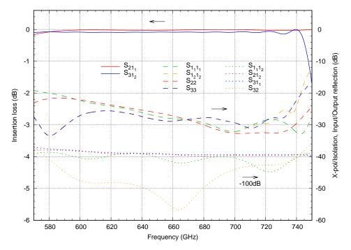
Figure 54: Simulated S-parameters of the Dunning OMT. The solid lines are the co-polar transmissions (i.e., the insertion losses), the dashed lines the return losses, and the dotted lines (offset by 100 dB) the cross-pol and isolation factors. Ports:  $1_1$  input H,  $1_2$  input V, 2 output H (straight), 3 output V (side). This is a simulation of the ideal structure; neither tolerances nor material losses were taken into account.
