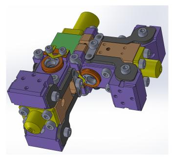
Figure 56: A view of the straw-man single-horn assembly from below, showing that, although there are some intersections, no vital parts (backpieces, magnet conductors, etc.) are interfering in a fundamental way.
