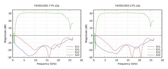
Figure 18: S-parameters of the two Yebes 4–20 GHz amplifiers (Y420G series) used in the 2SB measurements, obtained at 5.5K physical temperature. Compared to the earlier upgraded 2–14 GHz amplifier (Y214G, see fig. 16), the crucial improvement for our purpose is in the input matching ( $S_{11}$ , red curves). Data courtesy of Observatorio Astronómico de Yebes.
