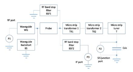
Figure 7: A block scheme representation of the main simulation elements for the layout of figure 6
