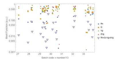
Figure 66: Merit function for automatically determined I-V curve parameters,  $R_n$ ,  $Q = R_j/R_n$ ,  $V_g$  and product of merit functions for  $R_n$ , Q,  $V_g$ ,  $DeltaV_g$  (open down triangles). The data is shown as function of batch code + batch number/13, i.e. all available SIS27xx batches are located between 27 and 28 on the horizontal axis.
