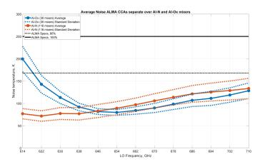
Figure 39: Average DSB noise temperature as in figure 38, but separated out for the  $AlO_x$  and AlN barrier mixers.
