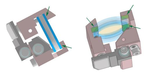
Figure 46: Views of the model drawing of the grid and its holder. The green arrows indicate where the shimming could be done.
