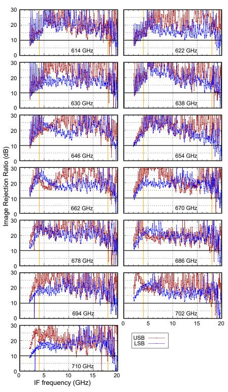
Figure 34: The Image Rejection Ratio as function of IF frequency for different LO frequencies. The thick lines at  $10\,\mathrm{dB}$  show the typical (current) ALMA spec.
