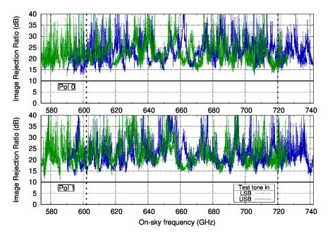
Figure 2: Image rejection ratio measured for the SEPIA660 receiver, as delivered. The LO settings are spaced by 8 GHz, and at each LO frequency the IRR is determined over the full 4–12 GHz IF band.
