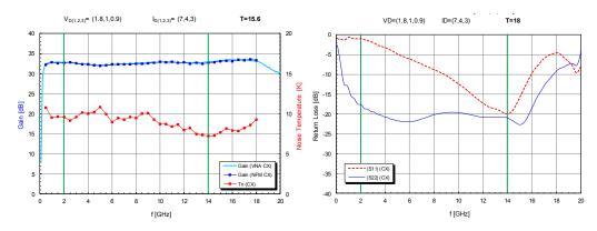
Figure 16: The gain and noise temperature (left) and the input and output matching (right) of the extended-band cryogenic 2–14 GHz LNA (Y214G 1027) used for the ultra-wide IF DSB measurements, at low temperature. Images courtesy of Observatorio Astronómico de Yebes.
