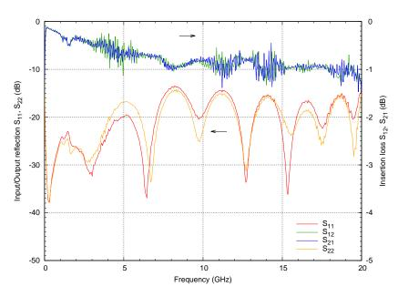
Figure 15: The S-parameters of the second new bias-tee (with conical inductor), after retuning, at room temperature. Now the input and output reflections are reasonably uniform at a -15 dB level
