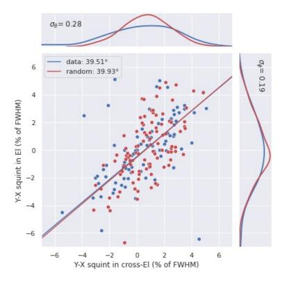
Figure 45: Comparison of the measured and simulated on-sky polarization beam squint. Blue dots are the data from Appendix B.2, while red dots are the results of the simulations with a random tilt with a gaussian distribution in the two orthogonal directions with  $\sigma_{\theta} = 0.28^{\circ}$  in one direction and  $\sigma_{\phi} = 0.19^{\circ}$ . Both measurements and simulation data have been fitted with a straight line to compare the direction of the beam squint in the sky.
