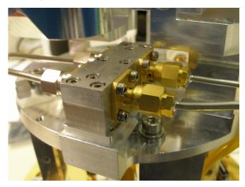
Figure 23: The 4-20 GHz IF quadrature hybrid mounted on an intermediate bracket to make it compatible with the earlier 4-12 GHz one. The two semi-rigid phase-matched cables on the right lead to the mixer (not mounted here yet).
