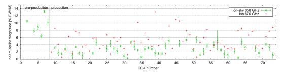
Figure 47: Comparison of the beam squints (as percentage of the beam FWHM diameter) of the deployed Band 9 receivers, derived from near field lab data (red +-es) and from on-sky measurements (green ×-es). Figure and data processing courtesy Neil Phillips, ESO.
