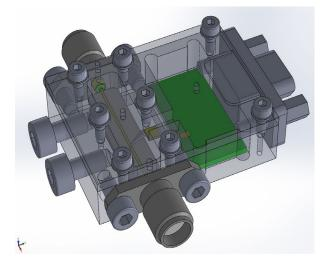
Figure 13: 3D rendering of the ultra-wide-band bias-tee. The IF cavity (left) contains a  $50\,\Omega$  microstripline coupled to two K-type connectors for input and output. A conical inductor couples in the DC voltage coming from the DC bias network board in the DC cavity (right). The six-point bias connection to the outer world is by MDM connector (far right). The large screws on the left are for mounting or additional heatsinking.
