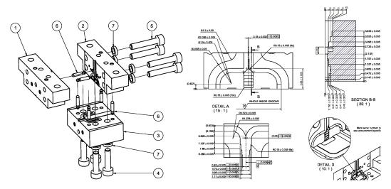
Figure 51: Exploded view of the Band 5 (163–211 GHz) OMT (left), and an impression of some of its fabrication details (right).
