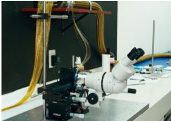
Figure 6. Mounting the 1300 optical fibres of the SOAR Integral Field Spectrograph at the LNA Optics Laboratory.
