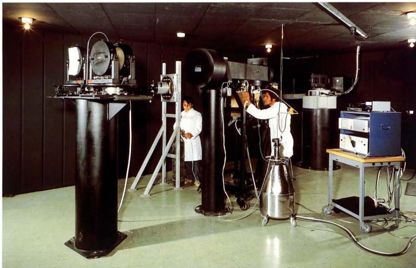
**218** Once every few years, the primary mirror of the 3.6-m telescope is stripped of its aluminium coating and then re-aluminized. During the operation, it is removed from the telescope and placed in a vacuum chamber in which the mirror surface is coated with a new layer of aluminium. In the photo we see the perfectly reflecting mirror after this delicate operation.
