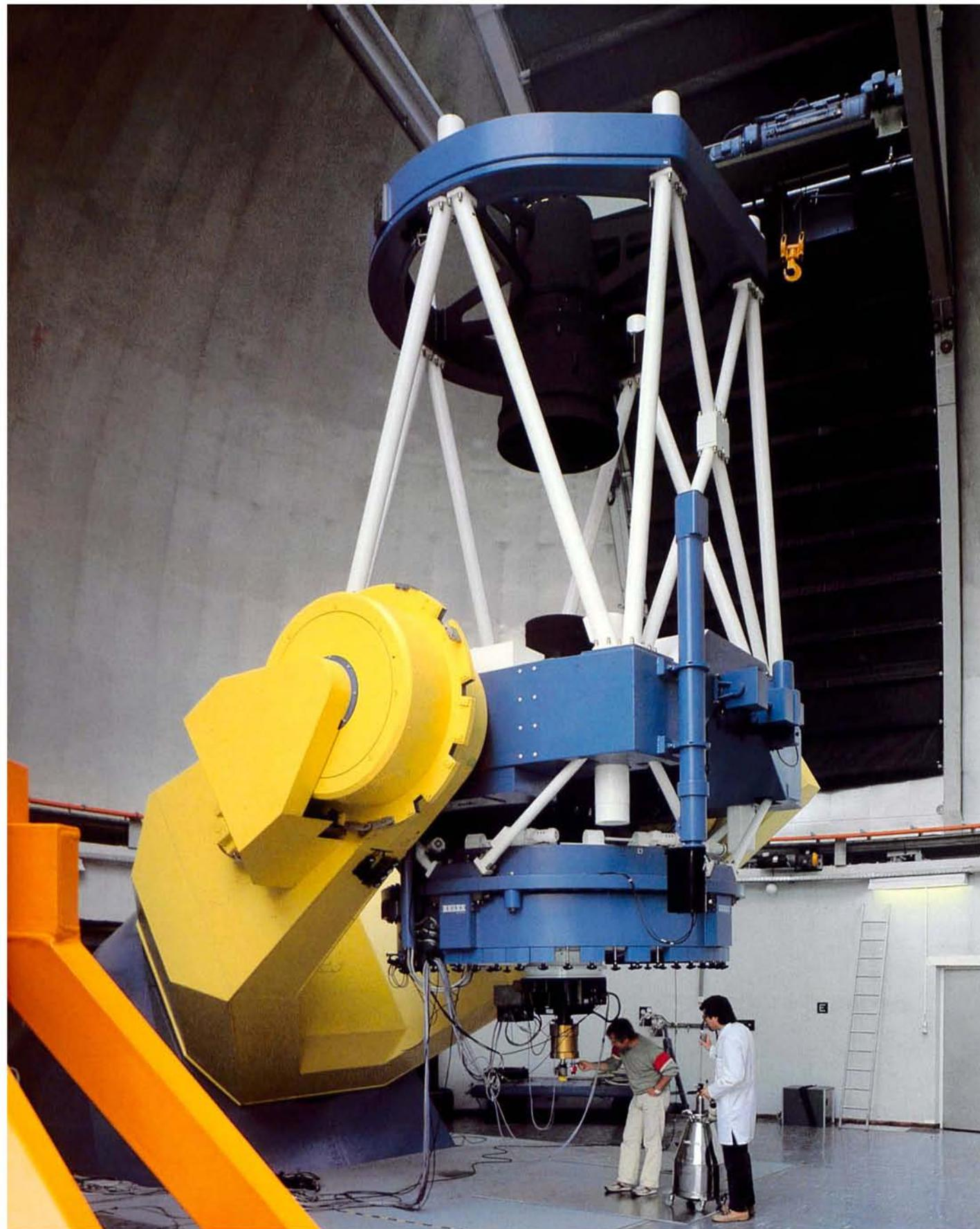
**225** Since being commissioned at the end of 1983, the 2.2-m telescope has enjoyed the status of the second-largest optical telescope in use at La Silla. It has been donated on long-term loan by the Max Planck Society in the Federal Republic of Germany. The equatorially mounted telescope was manufactured by M.A.N. and Carl Zeiss. It has taken some pressure off the 3.6-m telescope and is used for similar astronomical programmes.
