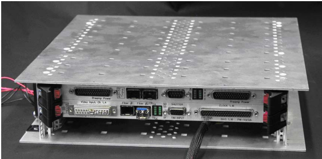
Figure 44 NGC prototype for a single Hawaii-2RG array in 32-channel mode containing NGC basic board with fiber communication, sequencer, bias and clock level drivers and AQ-32 board with 32 16-bit ADC's. Top: front side. Bottom: back side.
