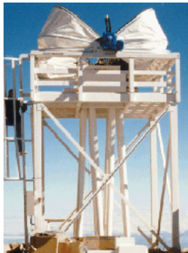
Figure 3: the automated ESO-DIMM at the VLT Observatory with its daytime protection enclosure at Paranal 2007.
