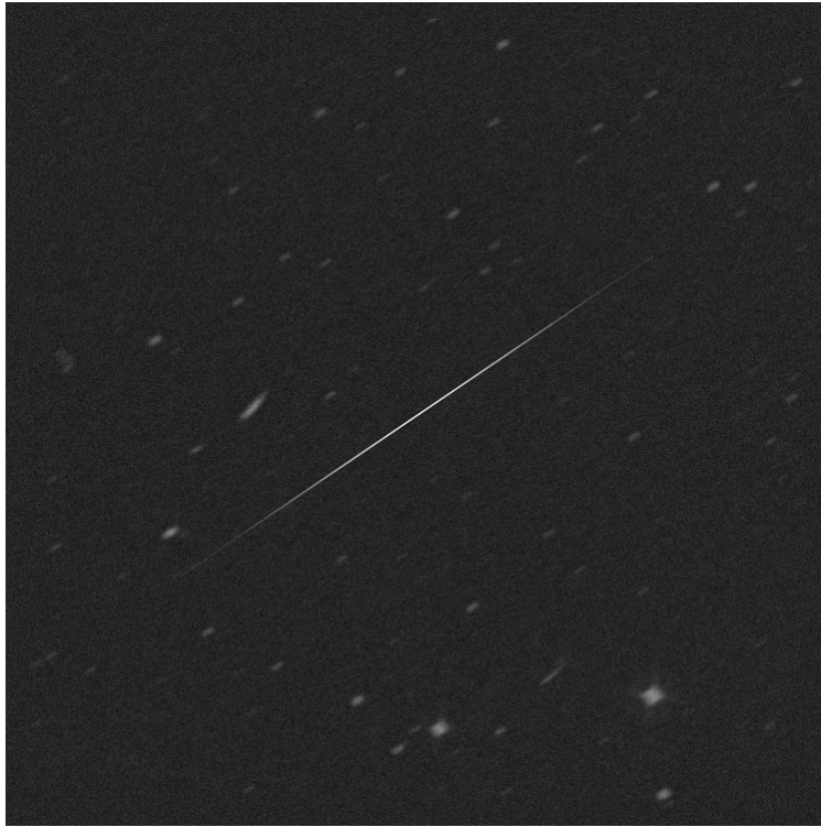
Fig. 5: VLT pointing close to zenith: alfa 00 00 00 VLT, delta -24 00 00, hour Angle 00 00 00. LGSM at La Montura, exposure 30 s, seeing 1.2 arcsec, sky background 19.5, field size: 750x750 pixels.
