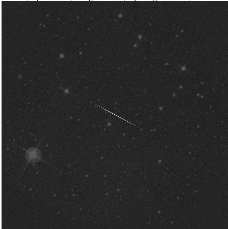
Fig. 6: VLT pointing to the pole, alfa 00 00 00, delta -90 00 00, hour angle 00 00 00. LGSM at La Montura, exposure 30 s, seeing 1.2 arcsec, sky background 19.5, field size: 750x750 pixels.
