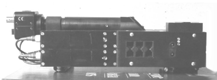
Figure 3. Photograph of the detector box. The buttons for manual control and the mounting flange are seen on the right, the two PMT modules and the viewer with guiding TV camera – on the left, the connectors to the RS-485 line – at the center. The length of the detector box is 21 cm.
