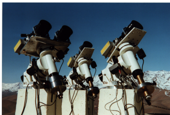
Fig. 1. View of the GSM instrument at La Silla. The central pier with two modules in differential configuration is seen on the left, the eastern module in the center and the southern module on the right.
